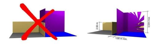
The back side of any building elements exceeding 2,50m high should be covered with a white scraped coton or a white paint in order to leave a clean appearance on these parts of the stand.
